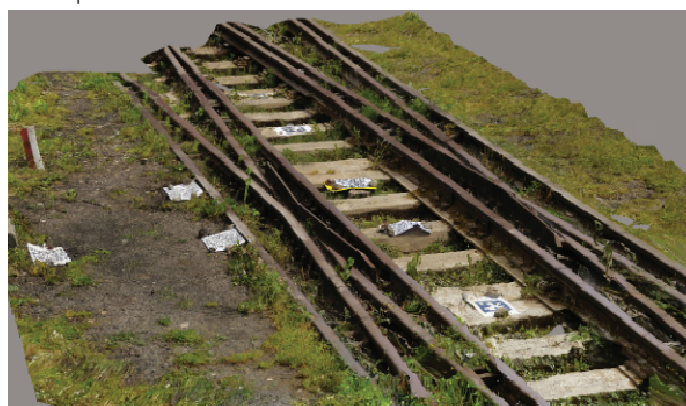
6. 3D model (from one measuring point) made in iTwin Capture Modeler
