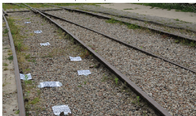
5. Example of QR codes and april tags location based on photo from point No. 1
