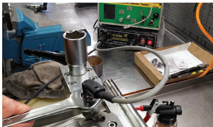
7. Adjustment of the air gap (GAP) in Siemens VDO Continental injectors Source: own study
