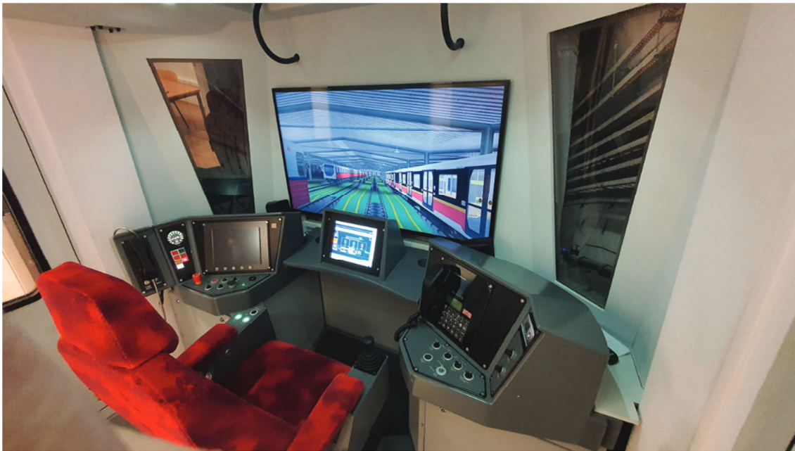
1. The interior of the Siemens Inspiro vehicle simulator cabin
