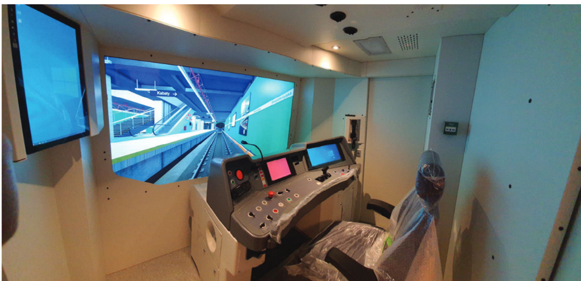
6. The interior of the Škoda Varsovia vehicle simulator cabin
