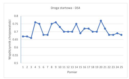
**9**. The course of variation of the friction coefficient determined for the surface of the runway marked DS4 at a speed of 95 km/h and with a water film
