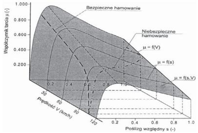
**2**. Spatial function of the friction coefficient depending on the speed and the size (degree) of slip [Sandecki 2017]
