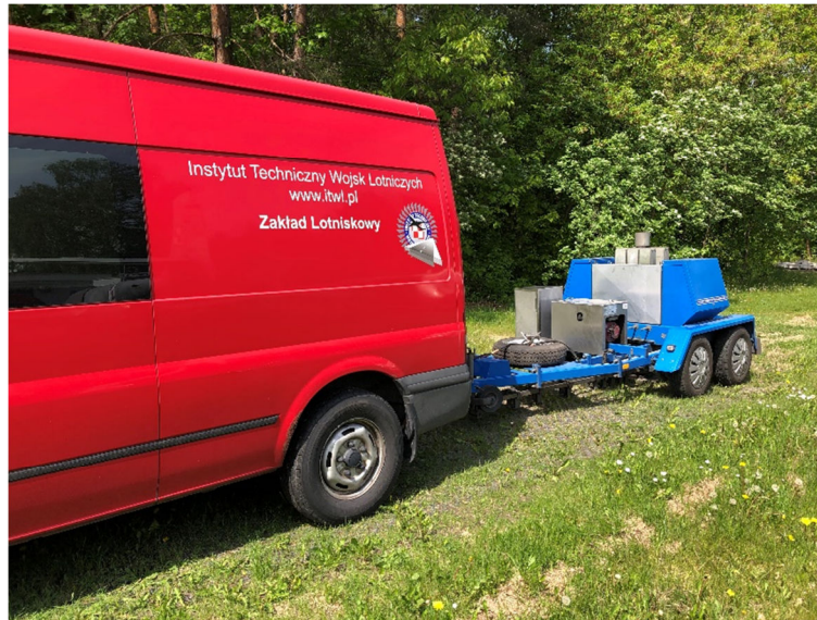
13. Measurement of bearing capacity with the HWD airport deflectometer
