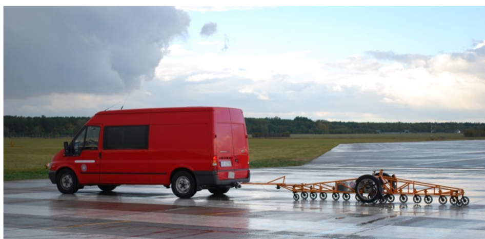
1. The planograph P-3z during evenness measurements
