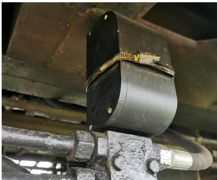
3. Mounting place of the transmitter on the WM-15A motor wagon
