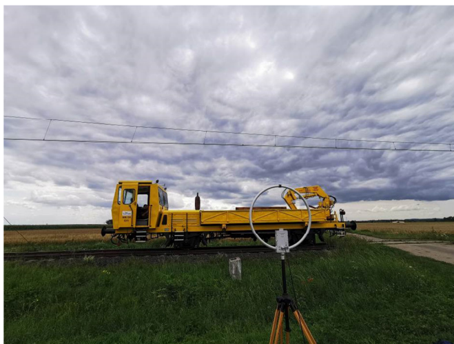
11. Stand for measuring the emission of radiated disturbances in the frequency band 150 kHz - 11 MHz
