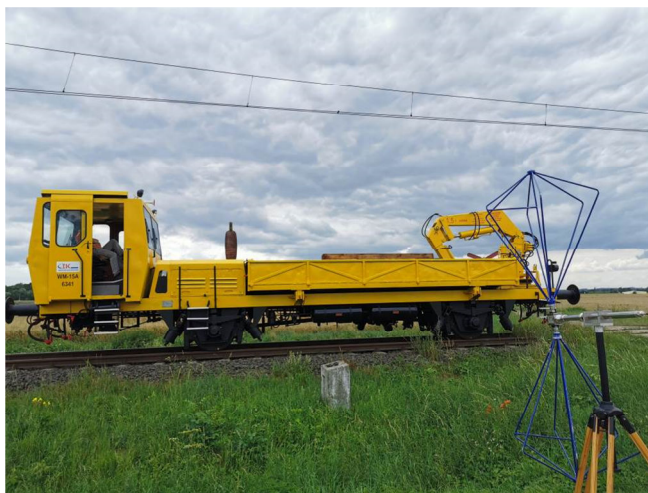
10. Stand for measuring the emission of radiated disturbances in the 30 MHz - 230 MHz frequency band
