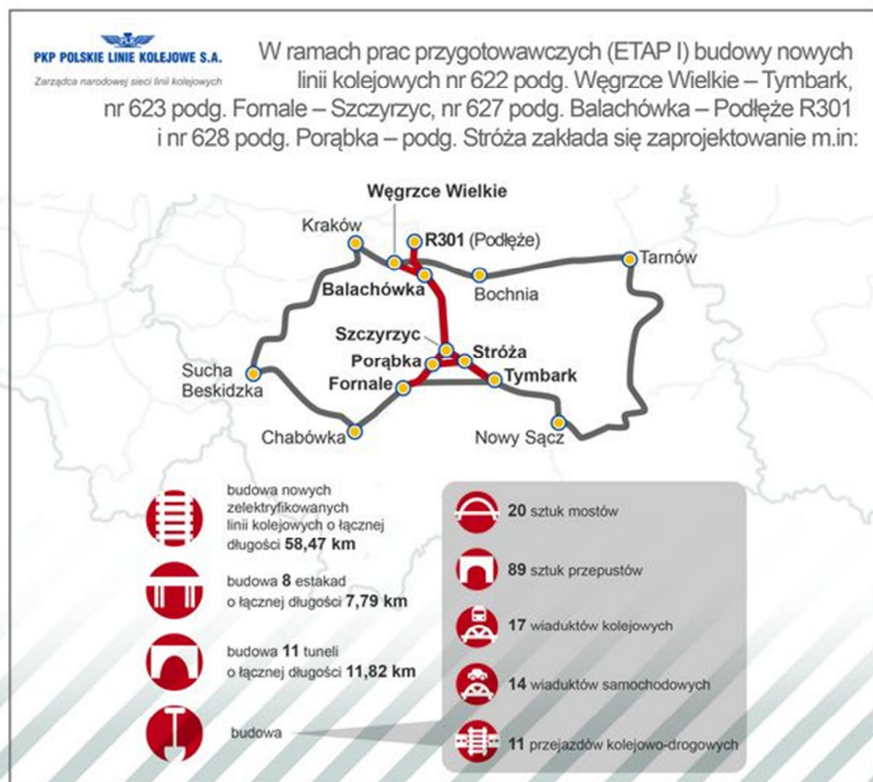
2. The material scope of construction of the Podłęże – Szczyrzyc/Mszana Dolna – Tymbark line. Source: [18]
