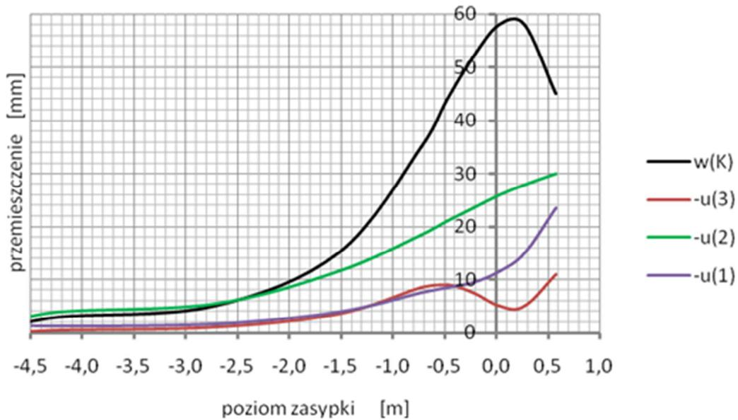
8. Changes in displacement of measuring points during the arrangement of the backfill
