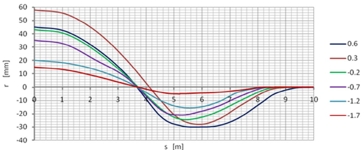
9. Lines of displacements in the radial direction of the circumferential strip of the shell
