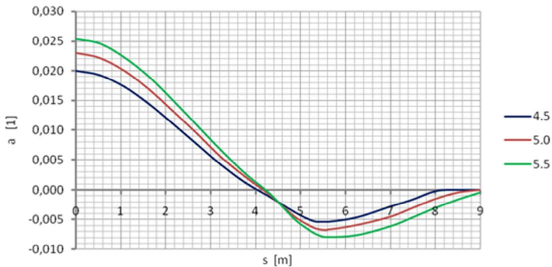
10. Lines of uplift influence as a result of FEM calculations. In the legend, the height of the shell  $H$ .
