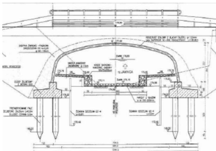
2. Supporting the shell on the foundation with the use of reinforced concrete piles
