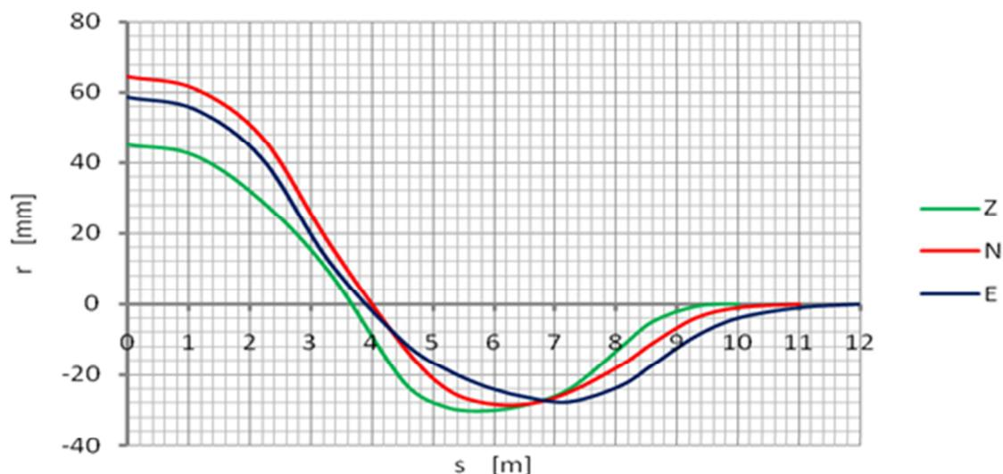
12. Displacement lines of the circumferential strip of the shell depending on the ground level
