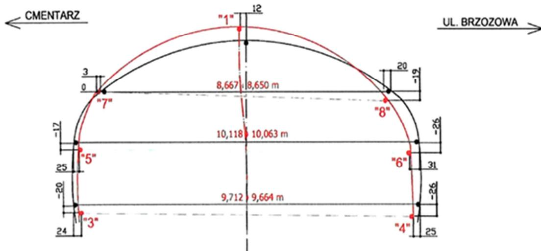
11. Diagram of the deformation of the circumferential strand of the shell after the surface treatment
