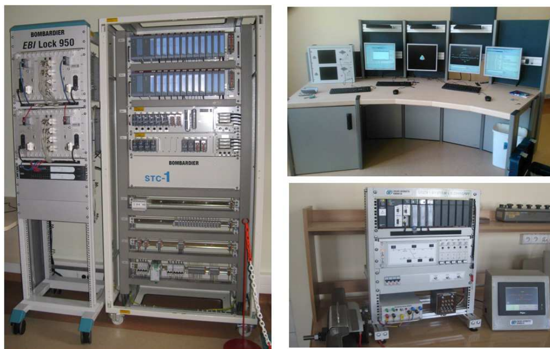
9. View of sample laboratories designed to: a) study the EbiLock 950 adjustment system of the Transportation Bombardier (ZWUS) Poland; b) execution of the trains on the ZSB 2000 configuration panel of Scheidt & Bachmann Polska; c) control of unchecked SKZR tracks manufactured by Z.A. KOMBUD Radom [4].
