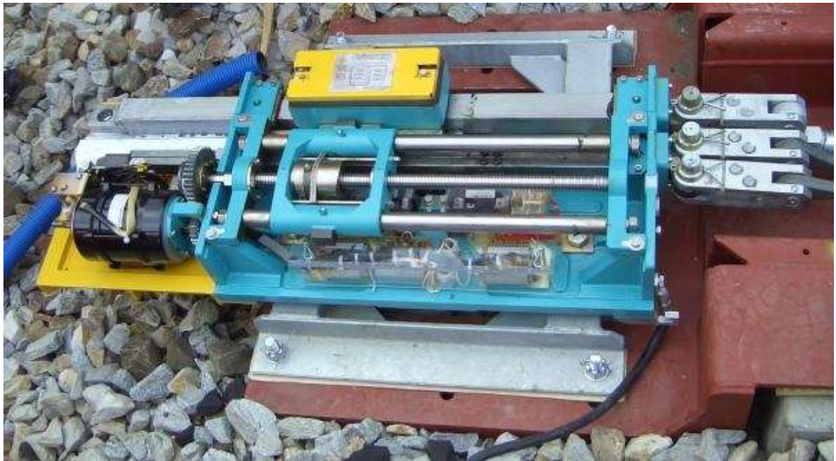
1. Construction of drive EEA 5
