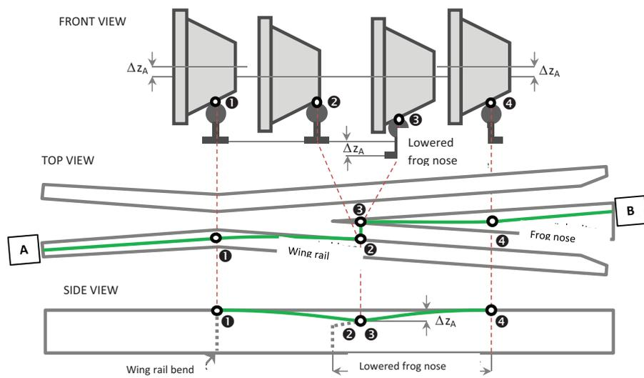
1. Constructional geometry (schematically)
