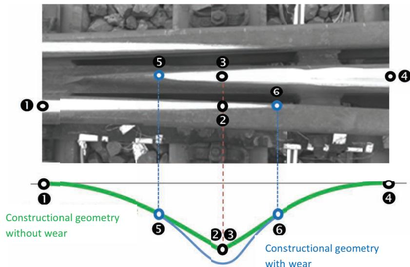
2. Wear geometry (schematically)
