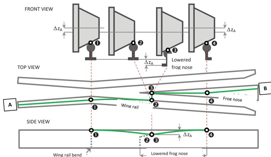
1. Constructional geometry (schematically)
